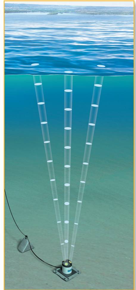
The Argonaut-XR measures water velocities at each of the profiling cells.
