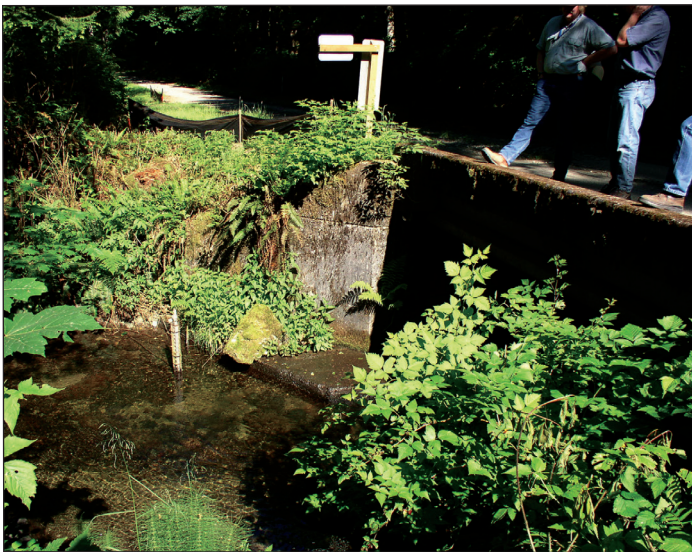
A turbidity sensor was installed in a tributary of the Cedar River watershed to monitor water quality conditions for Seattle, Washington.
